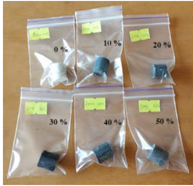
Figure 2. Made samples of fluoroplastic F4 and composites with graphitized dust
