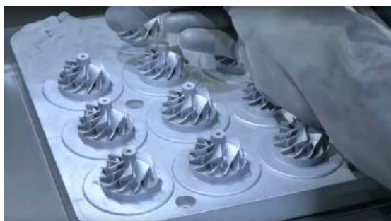
Fig. 8. Cleaning of the printed centrifugal impellers from powder
