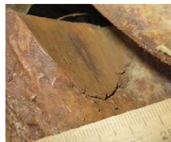
Fig. 2. The nature of the destruction of the working surface of the drive wheel
