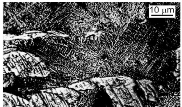
**Fig. 4.** Nucleation and growth the second eutectic  $\gamma\text{-Fe}$  phase (austenite) on the terrace of primary  $\text{Fe}_3\text{C}$  crystal
